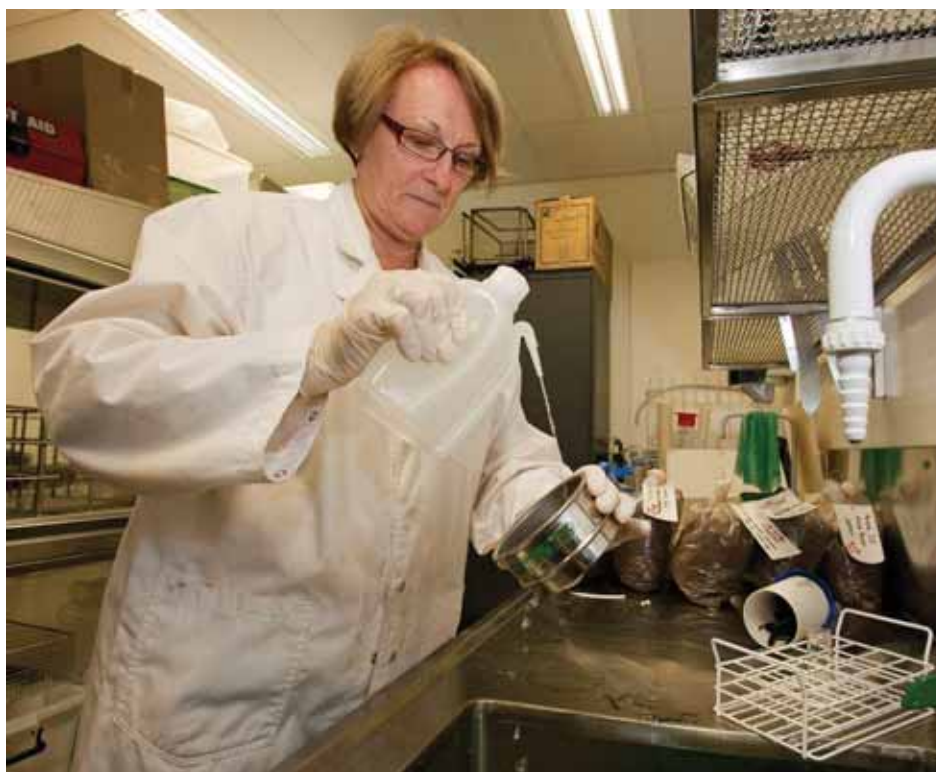
Image 1 Jennifer Cobon extracting nematode eggs on a 38 \mu\text{m} sieve.
