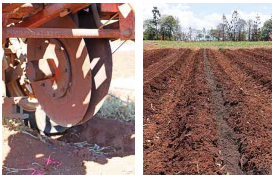
Image 20. Double discs used to create v-furrow (right) and compost amendment in v-furrow (right)
