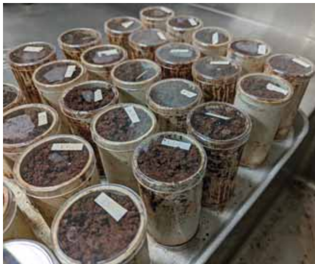
Image 23 Inoculated core assays incubating in the laboratory.
